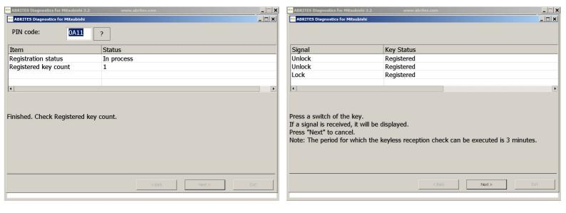
The PIN code of the vehicle will be automatically generated once the procedure is started. Before proceeding with the key programming function, you should make sure that you are using the correct transponder chip. The transponder in the key should be HITAG (PCF7936). It should be configured to work in Password Mode. The transponder can be configured by using the "Tag Key Tool" software.
